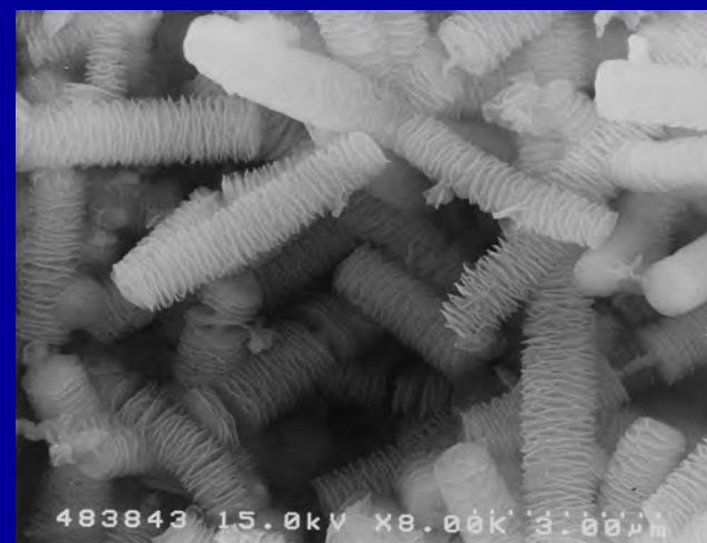
Fig. SEM images of ZnO nano particles prepared by heating \text{Zn}^{2+} -HMT aqueous solution at 95°C for different reaction time.
