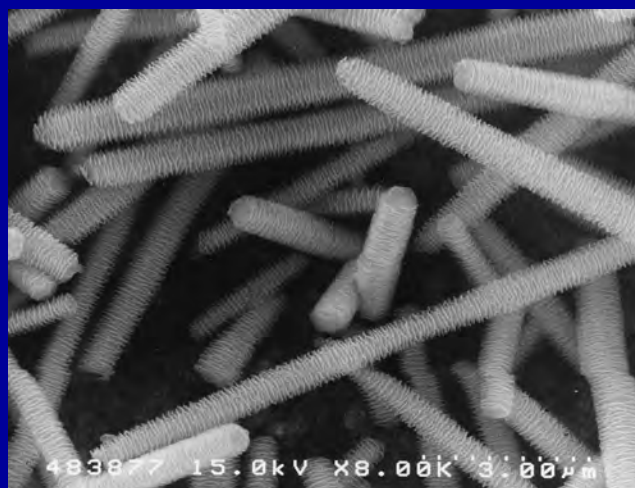
Fig. SEM images of ZnO nano particles prepared by heating \text{Zn}^{2+} -HMT aqueous solution at 95°C for different reaction time.
