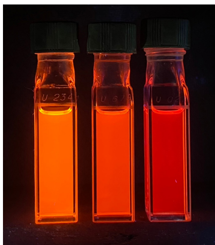
Figure S5. Photograph of AIS/Ag–In–Ga–S/Ga–S core/graded shell QDs under 365-nm UV irradiation, synthesized at In–S growth temperatures of 180 °C (left), 200 °C (middle), and 220 °C (right).
